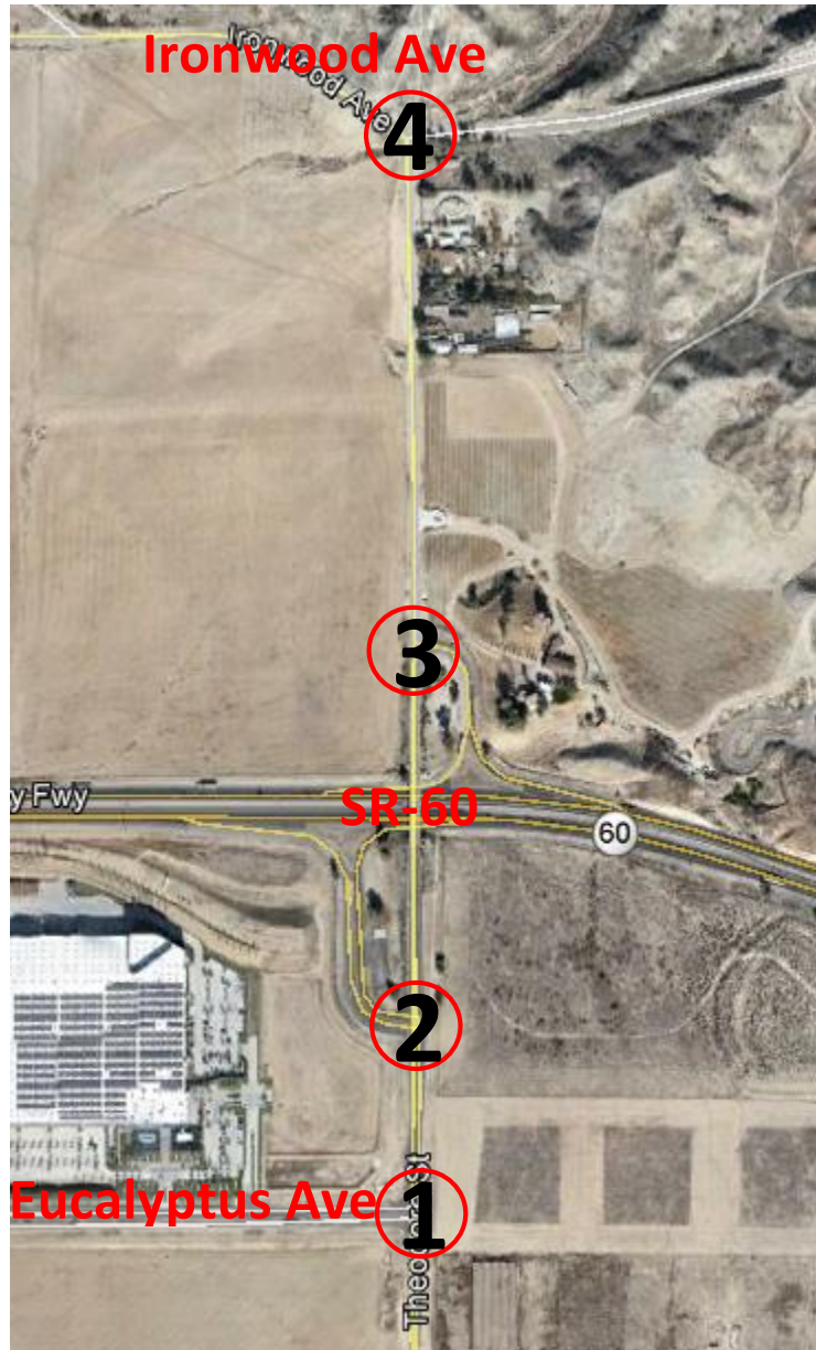
Figure 1. Overview image of the intersections under consideration, numbered 1-4. The CFI alternative replaces the intersections numbered 2 and 3.
